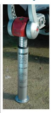
You can buy a noseweight gauge to check your unit's true noseweight before each trip or use a piece of wood (such as a section of broom handle) along with a set of bathroom scales to do the same job.
