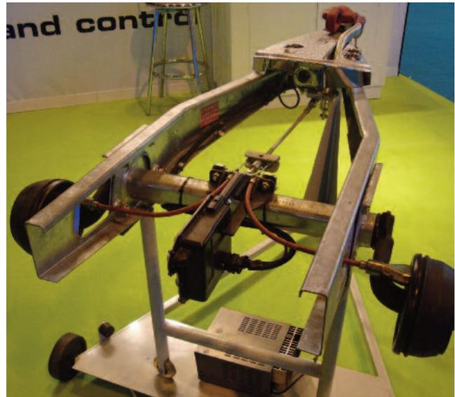
AL-KO introduced the ATC (Automatic Trailer Control) system – shown in demonstrator form above – for its chassis in 2007, and the idea has taken off with many manufacturers fitting it as standard on some models. BPW has a similar system called iDC (Intelligent Drive Control) for use on its own chassis, such as those used by Elddis in the UK. Practical testing has proved that both these systems are effective in maintaining stability under severe conditions.
