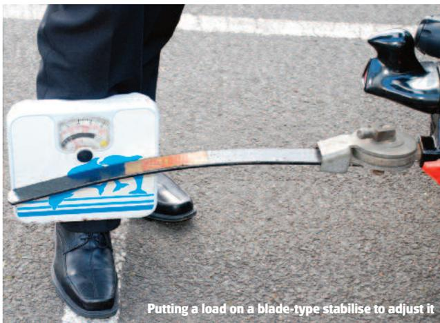
Putting a load on a blade-type stabilise to adjust it
