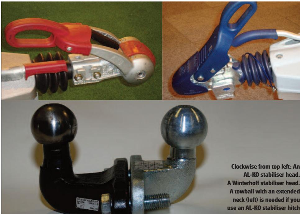
Clockwise from top left: An AL-KO stabiliser head. A Winterhoff stabiliser head. A towball with an extended neck (left) is needed if you use an AL-KO stabiliser hitch
