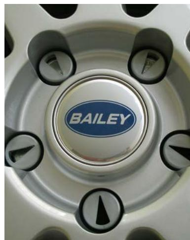
Left: It's a good idea to regularly check the wheel fixing bolts – indicators like these will help show if any are loose. Image courtesy of Milenco.
