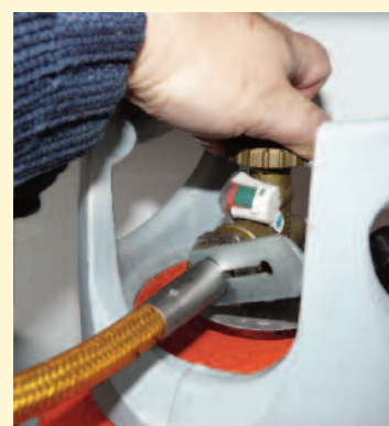
Make sure the valves on the top of gas cylinders are closed or the regulators disconnected and caps fitted
