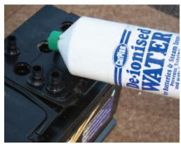
If the electrolyte level falls in the cells, each one should be topped-up with de-ionised water
