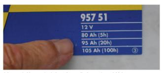
A battery's Ah capacity is based on a discharge time of 20 hours; some quote for three discharge periods
