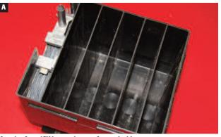
A casing for a 12V battery is manufactured with separate compartments
