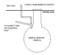
Suitable cesspools are fibre glass and should have a suitable lining to resist any attack by the chemicals in the waste. Alternatively a brick or concrete chamber with a suitably chemical resistant lining and covers may be used. Venting should be fitted. A 600 gallon (2700 litre) cesspool should be adequate to allow one empty / season. Note: This is dependent upon the amount of water discharged by flushing and rainwater ingress.
